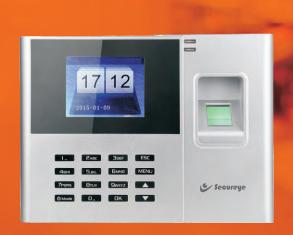
S-B251CB is a 7.11cm (2.8) TFT screen Time Attendance Terminal. TCP/IP and USB Host make data management extremely easy. Most importantly, the built-in backup battery can eliminate the trouble of power-failure. With elegant appearance and reliable quality, you can get the best from it
